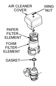
Figure 23. Engine Air Filter
